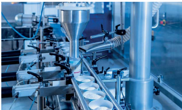
Filling of cardboard cans. Such cans are increasingly being used in the food industry as more sustainable replacements for aluminium ones.
