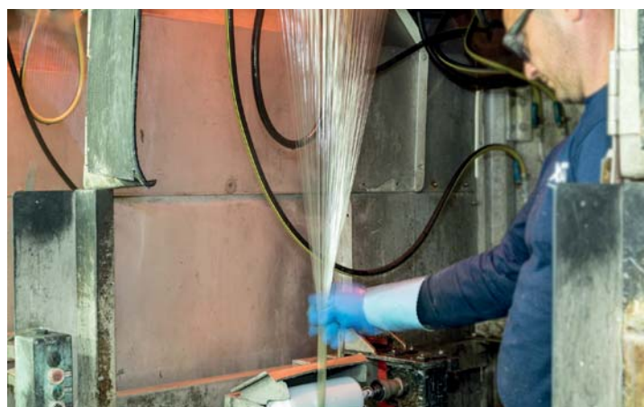
LANXESS using waste glass at its glass fibre production facility in Antwerp, Belgium. (Photo: LANXESS AG)
