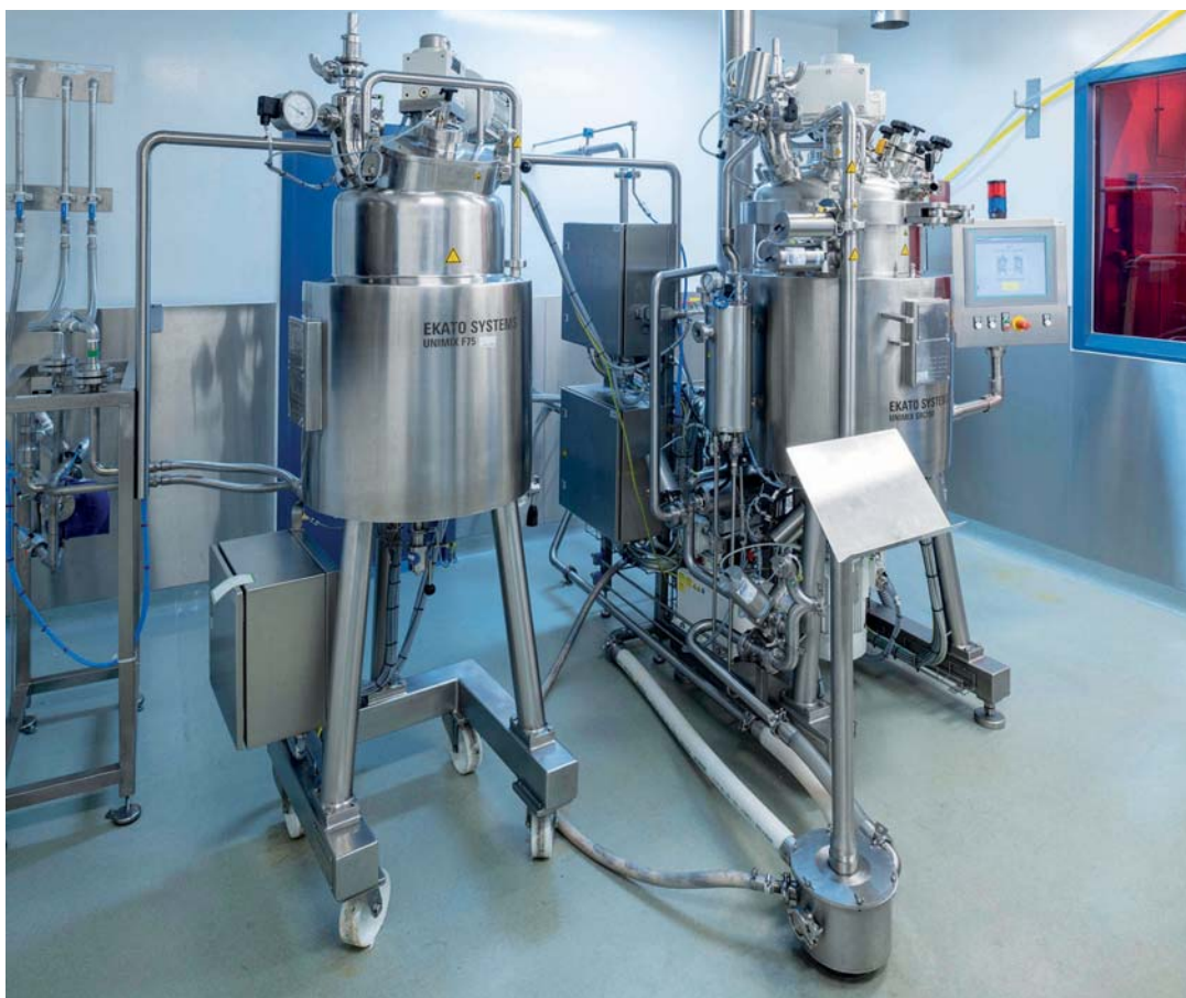
The Ekato 150L Mixer Homogenizer is used for semi-solid manufacturing from 40 to 150L employing either high or low solid-liquid shear and comprises a jacketed main vessel and 75L side vessel under PLC temperature control. There is also a clean-in-place (CIP) system to ensure safe and highly-efficient cleaning of the equipment.
