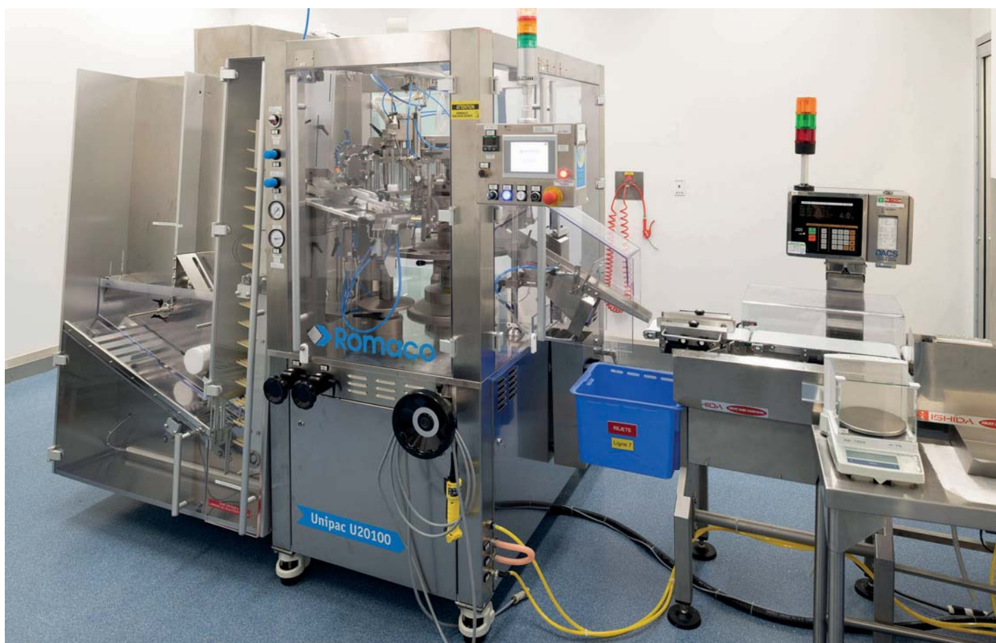
The Romaco Unipac 20100 Tube Filler is also used in semi-solid manufacturing, specifically to fill PVC, laminated and metal tubes with topical products in quantities ranging from 2-250g.
