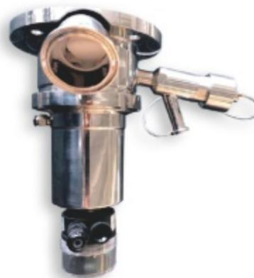
VALVOLA ASETTICA DI FONDO PNEUMATICA IN SMO 254 TAMPONE IN TFM 1705 PTFE CON ATTUATORE IN INOX E BOX FINECORSO INDUTTIVO - CORPO ASPORTABILE CON CONTROLLO FLANGIA SALDATA AL TANK CON PRELEVA CAMPIONI MODELLO AS2 PNEUMATICO INOX ESD/UTC SALDATO AL CORPO PRINCIPALE DELLA VAF
