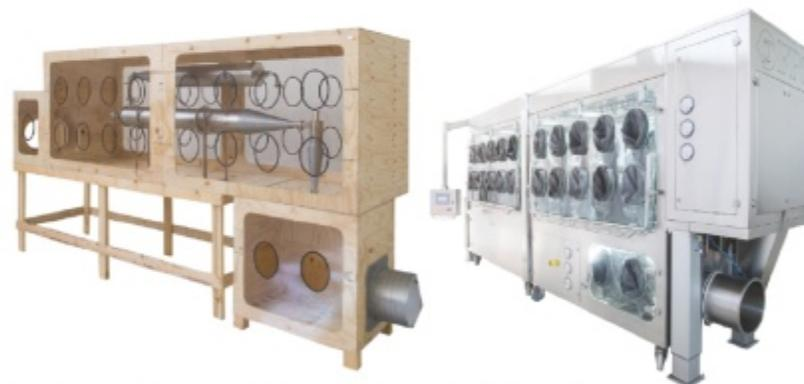
**MOCK-UP AND FINAL PROJECT OF ISOLATOR FOR SPRAY DRYER AND MICRONIZATION**
