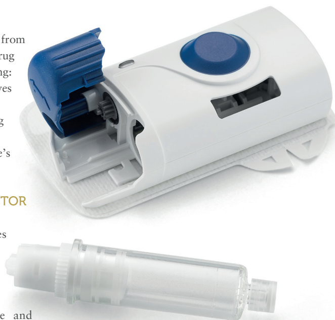
Figure 3: West's SmartDose® 3.5 injector used by Amgen for their Pushtronex® system.
